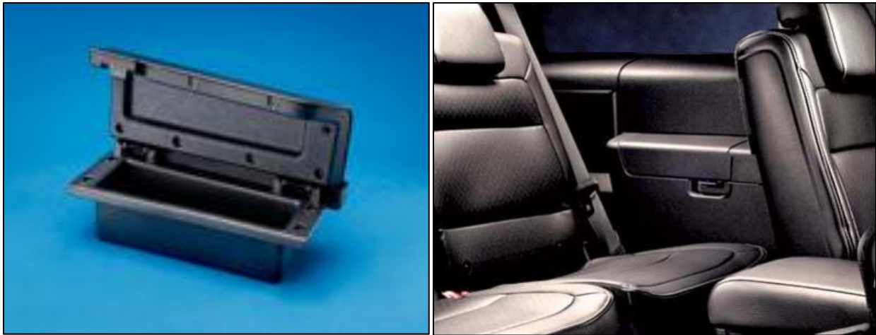
Figure 10: Wheat Straw/Polypropylene Storage Bin and Cover Liner for the 2010 Ford Flex
