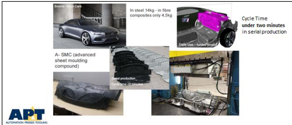
Figure 32: A-SMC Components Formed in Less than 2 Minutes
