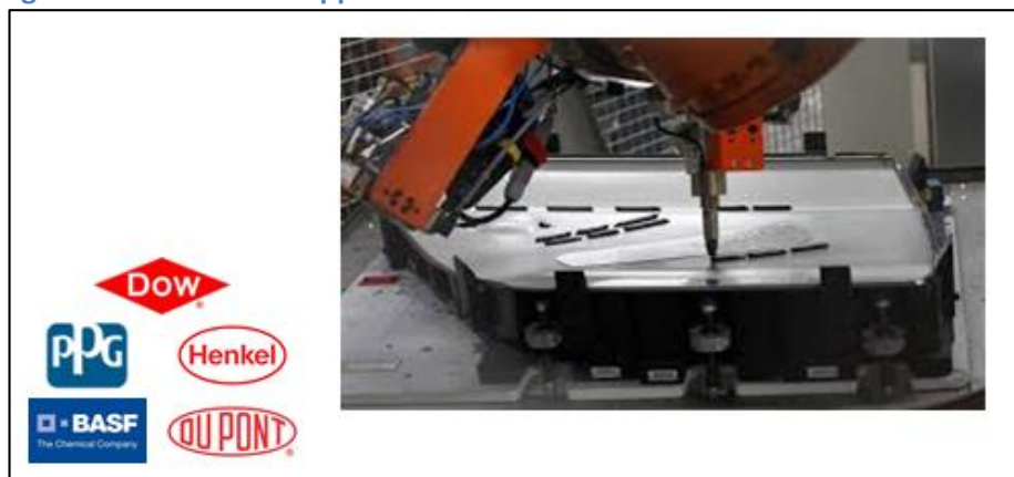
Figure 19: Automated Application of Structural Adhesives
