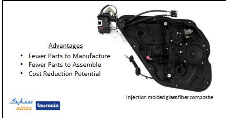
Figure 44: Thermoplastic Sealed Door Module (Advanced Consideration)
