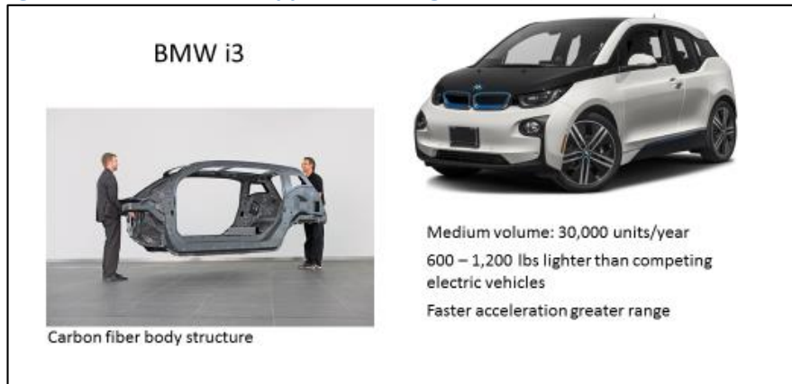
Figure 36: Carbon Fiber Application Progression (BMW i3)
