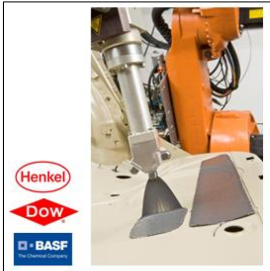
Figure 23: Automated Application of Liquid Applied Sound Deadener
