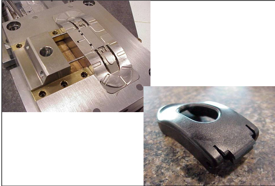
Figure 45 – Conformal Cooling Tool for Fiat and First Shot (CRF)
