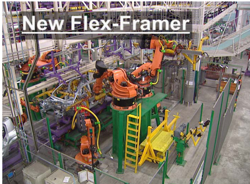
Figure 13 – Renault Flexible Robotic Body Framing Cell
