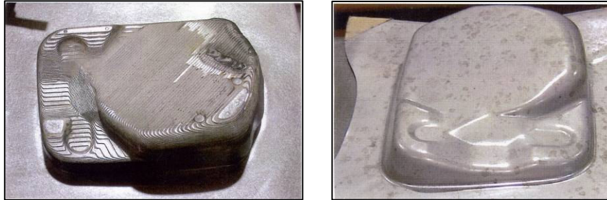
Figure 36 – Laminated Die (Before Final Machining) and Drawn Part
