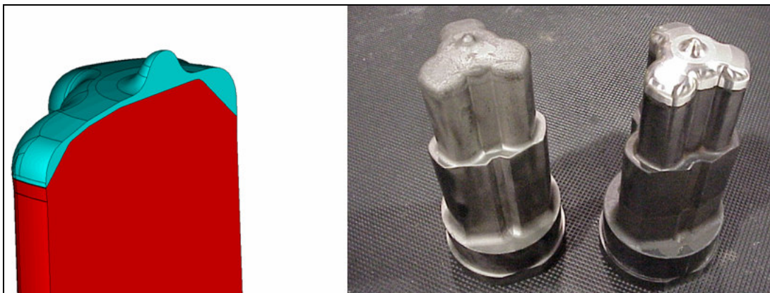
Figure 44 – Laser Deposition Tool Coating
