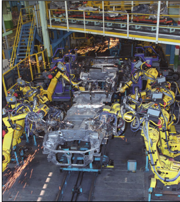
Figure 9 – Honda Underbody Re-spot Line
