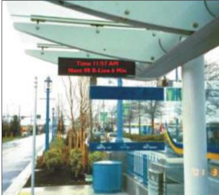
FIGURE 11: REAL-TIME PASSENGER INFORMATION DISPLAY AT BUS TERMINALS 139
