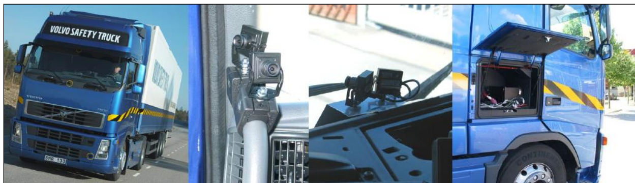
FIGURE 25: VOLVO FH12, CAMERAS, AND LOCATION FOR SYSTEM INSTALLATION IN SIDE COMPARTMENT 386
