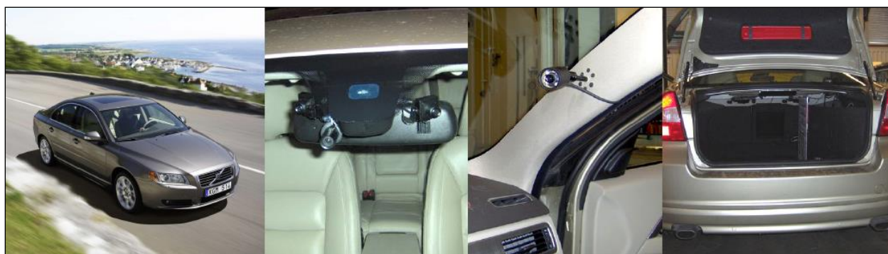
FIGURE 26: VOLVO S80, CAMERAS, AND LOGGER INSTALLATION IN LUGGAGE COMPARTMENT 387
