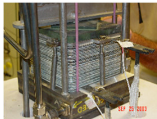
Stack sealing in progress
