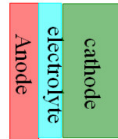
Cathode supported cell
