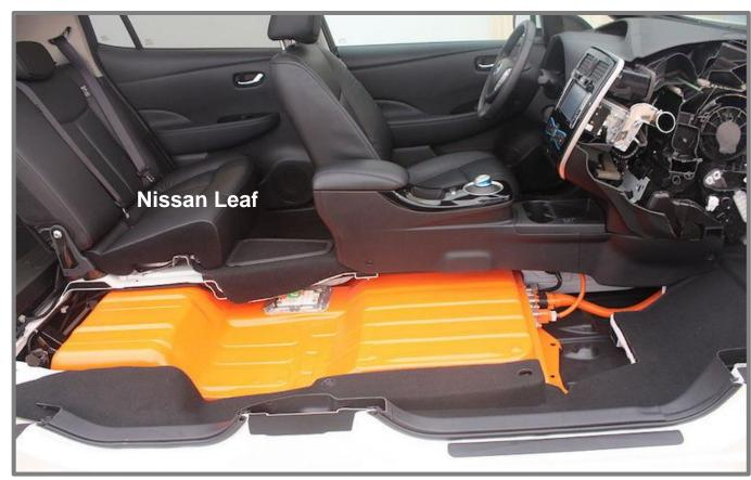
Passenger sits – literally – on top of the battery cover Importance of Fire protection is evident
