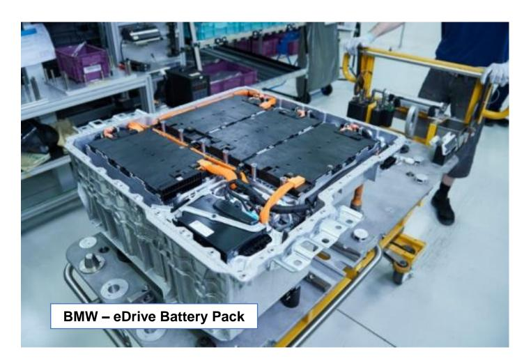
Example of 3D Cast aluminum tray and cooling system
