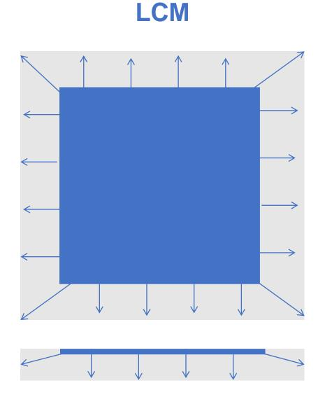
Resin Flow/Fiber Impregnation (during Mold Closure)
