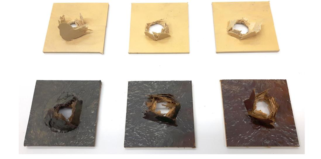
EPONOL 06921 SMC retains >65% of its strength and impact resistance even after full fire exposure.
